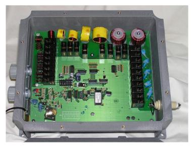
Designed and produced in the USA by SEA, an industry leader in high technology communications equipment, the SEA 1612C automatic MF/HF tuner combines the sophistication of advanced microprocessor techniques with high order practicality and operational reliability. The SEA 1612C is housed in a weatherproof molded case designed to withstand rugged environmental conditions encountered aboard ship while mounted on the external weather decks.
