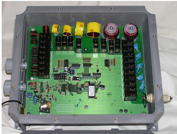
Designed and produced in the USA by SEA, an industry leader in high technology communications equipment, the SEA 1612C automatic MF/HF tuner combines the sophistication of advanced microprocessor techniques with high order practicality and operational reliability. The SEA 1612C is housed in a weatherproof molded case designed to withstand rugged environmental conditions encountered aboard ship while mounted on the external weather decks.
